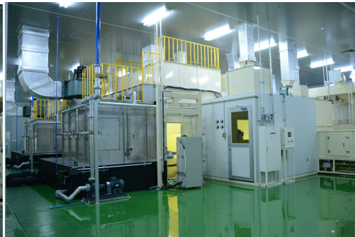
Water curtain booth with paint mixing room.
